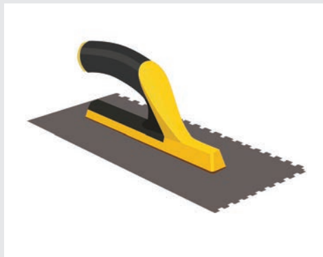
TROWEL FOR THE SLAB
