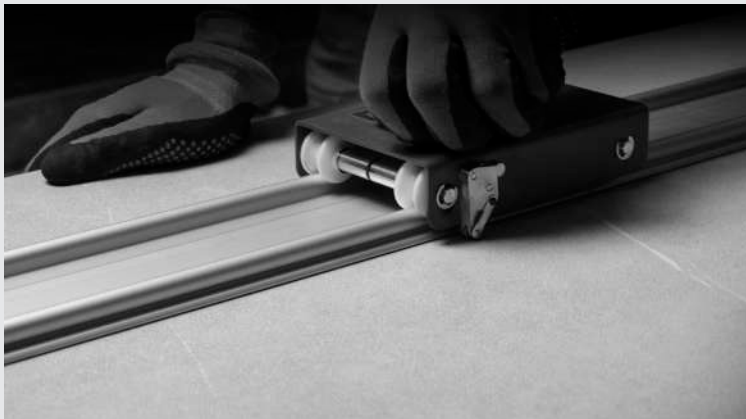
CUTTING DETAIL WITH GUIDE ON SLAB
